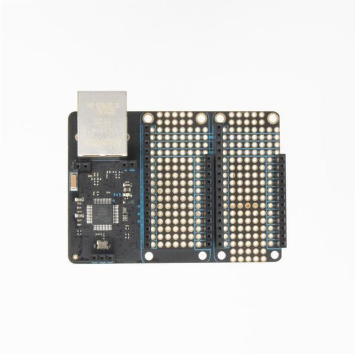
The Ethernet FeatherWing is the fastest way to add wired connectivity to your Argon, Boron, or Xenon and turns any Particle Mesh developer kit into an Ethernet gateway. Based on the WIZnet W5500 chip, this side-by-side FeatherWing maintains great RF performance even while adding Ethernet connectivity to any Particle Mesh device.
