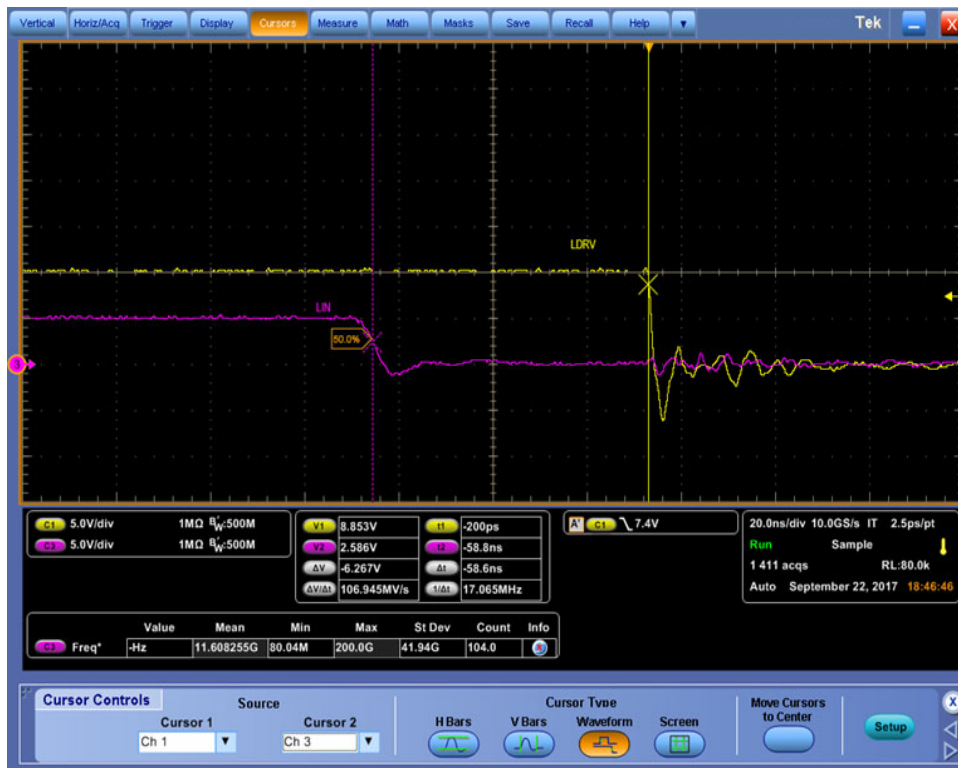
Figure 31. Low Side Turn-Off Propagation Delay (NCP51530A)
